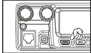
2. To turn the transceiver off, again press and hold in the **PWR** key for one second.
